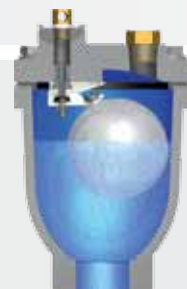
The valve will remain in closed position until it detects air pockets.
