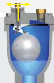
The valve will expel the air accumulated in a conduction when it is pressurized and in service.
