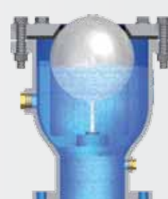
The valve is permanently closed until there is a detection of depression.
