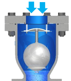
Air intake into the pipeline in the event of draining or pipe rupture
