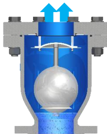
High-capacity air discharge during pipeline filling
