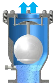
Discharge of large volumes of air during filling
