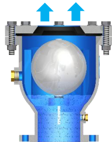
Large-volume air discharge during filling.
